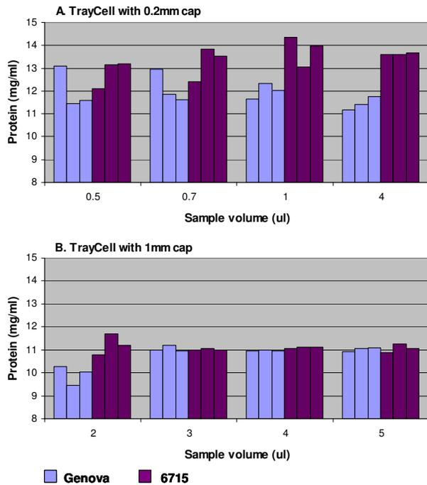
**Figure 2:** Protein concentration determined using various sample volumes in the TrayCell with A. the 0.2mm cap and B. the 1mm cap.
