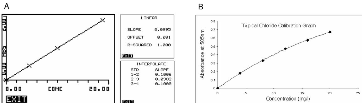
**Figure 1:** Example standard curves produced (A) by the model 6315 and (B) by plotting absorbance data of standards using Excel.
